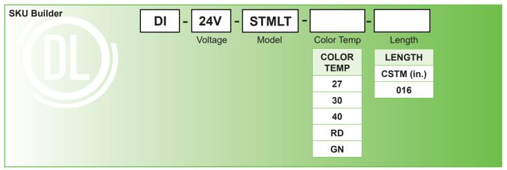
Example: DI-24V-STMLT-30-016 = Diode LED, 24 Volt, STREAMLITE™, 3,000° CCT, 16.4 foot spool.
